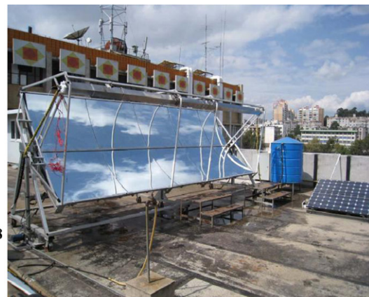
1. Trough Concentrator 2. Receiver 3. Storage tank 4. Pipe 5. Pump 6. Connecting rod 7. Supporter 8. Push rod.
