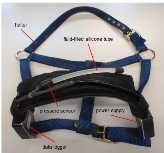
Fig. 1. Specifics of the automated measurement system (“RumiWatch”), integrated in a commercially available horse halter.
