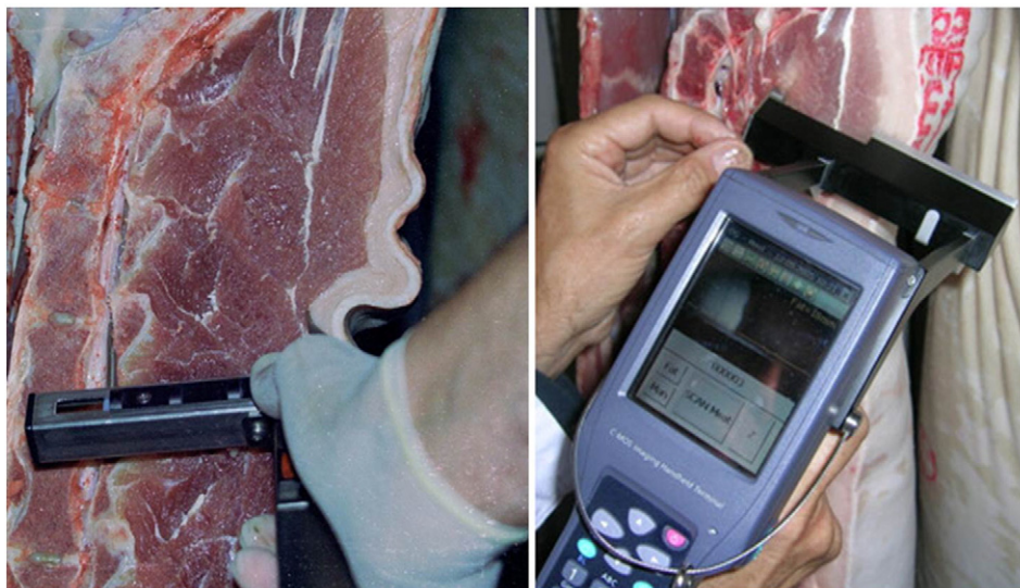
Fig. 2. ZP measurements with the electronic callipers MD02 (left) and Optiscan-TP © (right).
