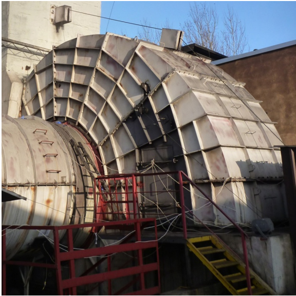
Fig. 1 – The steel casing of the centrifugal fan used for mine ventilation.
