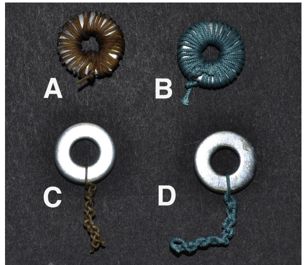
Fig. 1. SAE #10 (13 mm) flat zinc washer and suture combination designs for Experiment 3: catgut-wrapped washer (A), polyester-wrapped washer (B), washer with 15 throws of catgut (C), washer with 15 throws of polyester (D).
