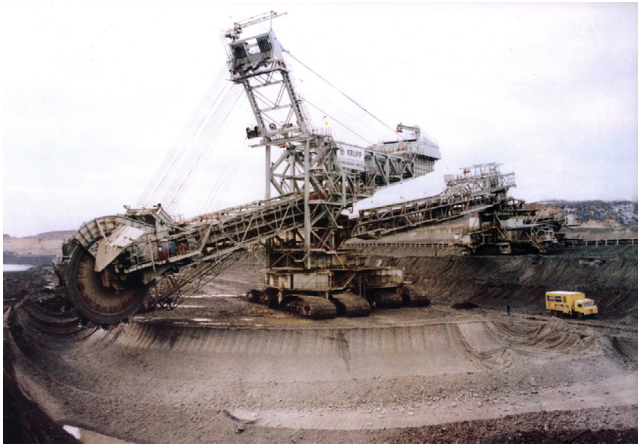
Fig. 1 – BWE SchRs 1760: total weight (with mobile conveyor) 3150 t, theoretical capacity 6100 m 3 /h.
