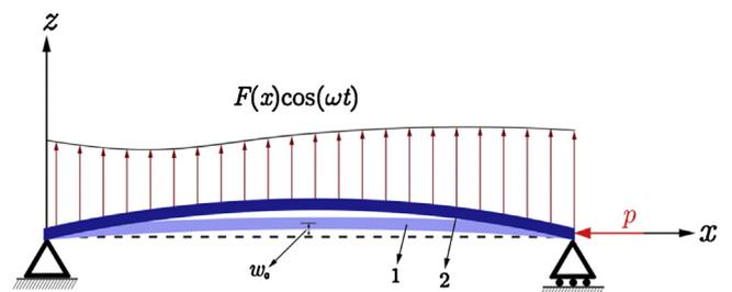
**Fig. 1 – Schematic representation of a microarch subject to a transverse distributed harmonic excitation force over the bent configuration (due to an axial load). Number 1 is the microarch before bending; number 2 is that after bending.**
