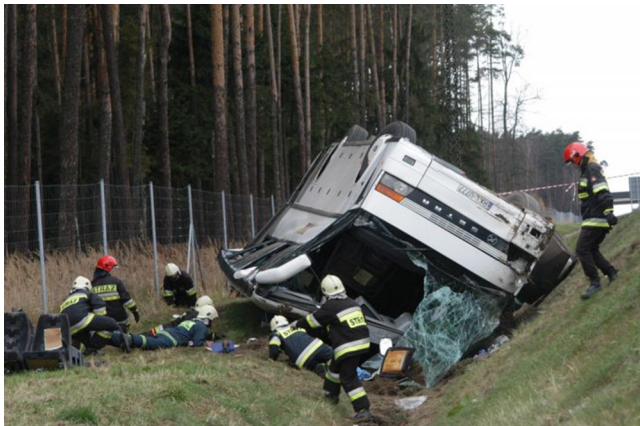
Fig. 1 – Infringed coach superstructure.
