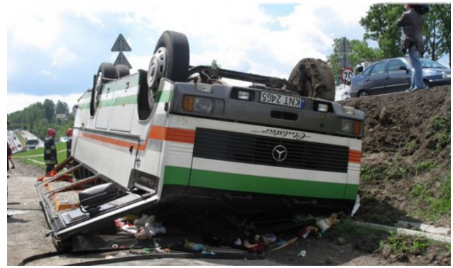
Fig. 2 – Significant deformation of side walls.
