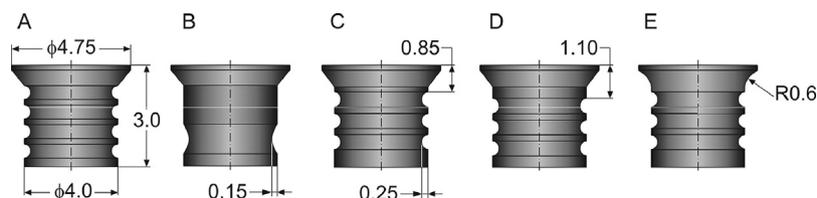
**Fig. 1 – Basic models (A and B) and rivet shape model's geometry changes (C-E).**
