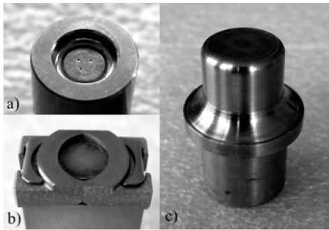
Fig. 1. conventional dies for clinch process: a) solid die, b) die with moving blades versus c) flat anvil as counter tool
