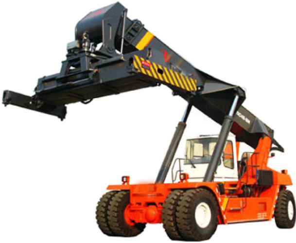
Fig. 1. Example of an off-highway working vehicle with a telescopic boom and a massive stacking gripper with its actuators [21].
