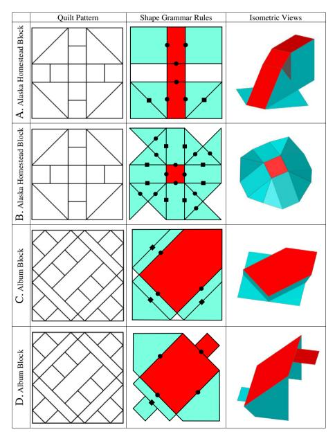
Fig. 1. Quilt-inspired concepts, including the established quilt pattern (including name), functional and three-dimensional shape grammar rules implemented (two-dimensional rules not shown for simplicity), and isometric views of the three-dimensional structures.
