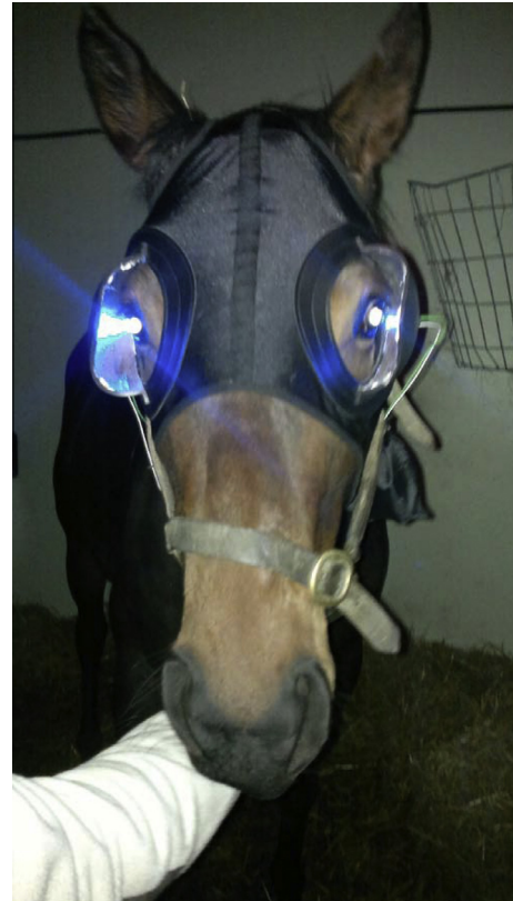
Fig. 1. Photograph of a horse wearing the light mask that provided light to both eyes. The light mask consisted of a modified full cup racing blinkers (Zilco) with a single blue LED (Kingbright 7.6 mm × 7.6 mm Super Flux LED Lamp L-7676CQBC-D Blue, GaN) fitted on the inside of each eye cup. The inner surface of the cup was covered with reflective aluminium foil to reflect light diffusely onto the eye. For the single eye light mask, only a single LED was fitted in the right eye cup and the right eye cup was covered over with a light-proof material.
