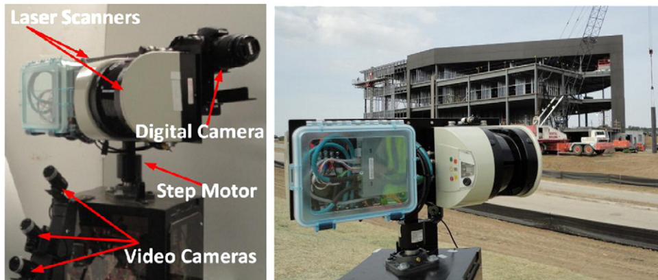
Fig. 2. Prototype data acquisition system (left) and a field data collection (right).
