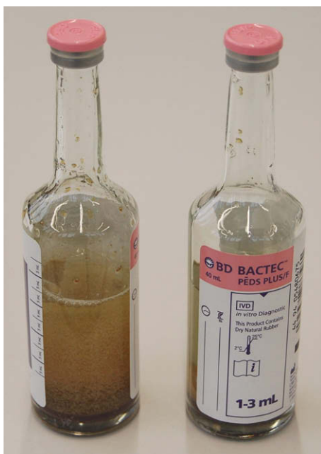
Fig. 2. Examples of BACTEC Peds Plus/F bottles. The resin granules can be observed in the medium as well as the fluorochrome-sensor at the bottom of the bottle.
