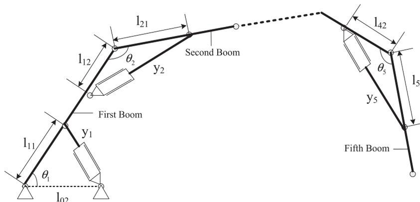
Fig. 1. Structural diagram of five booms.
