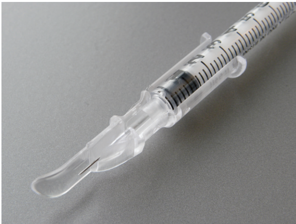
Figure 0. Prototype intradermal adapter attached to a syringe with a 29 gauge, ½-inch needle, as used in this study.
