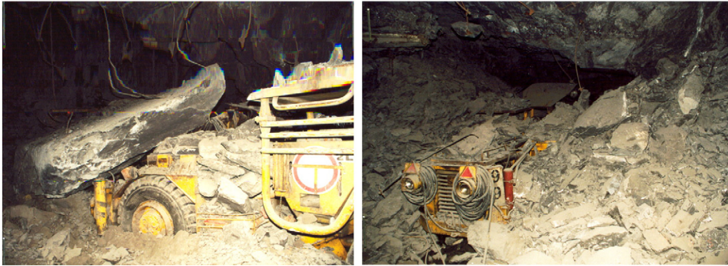
Fig. 1. Protective structure saved mining machine operator's life in KGHM PM S.A. O/ZG LUBIN — rockburst on 04.08.2003, rockburst energy: E=190\,000 kJ.
