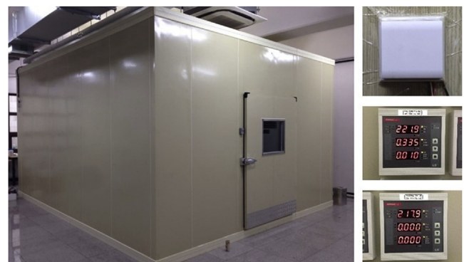
Fig. 1. Building Integrated Control Test-bed (BICT) used in the development of the occupancy prediction model.
