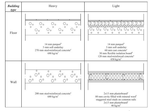
Fig. 1. The construction drawings of the floor and walls used between dwellings in the two *building types*. Approximate densities [kg/m<sup>3</sup>] of the materials: <sup>a</sup> 2500 <sup>b</sup> 700 <sup>c</sup> 2000 <sup>d</sup> 50 <sup>e</sup> 700 <sup>f</sup> 30.
