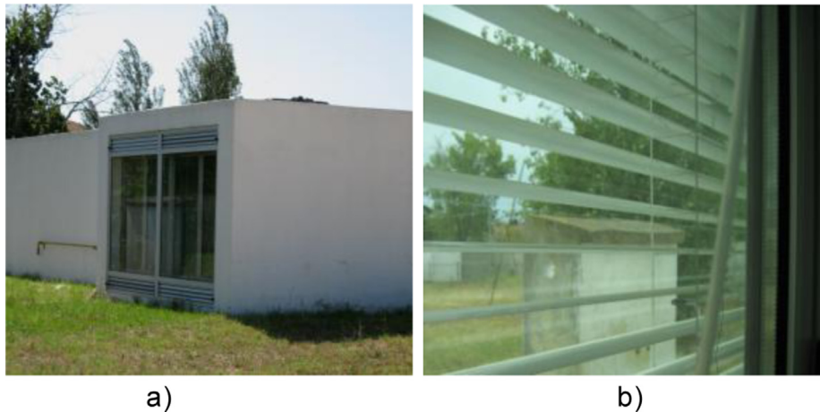
Fig. 1. Test cell (a) and fenestration system (b) used in the experimental study.
