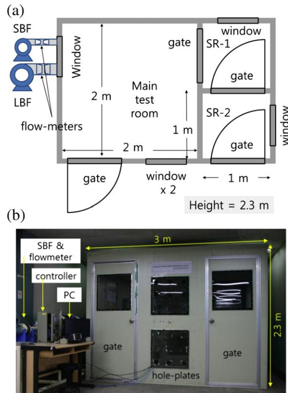
Fig. 1. An improved air tightness test room for the steady pressurizing method; (a) a schematic of the experimental test room (SR: supplementary room, SBF: small blower fan, LBF: large blower fan), (b) a photo of the experimental test room.
