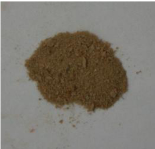
Fig. 1. Photograph of test powder containing house dust mite and cat allergens at a concentration of 10% of the total mass.
