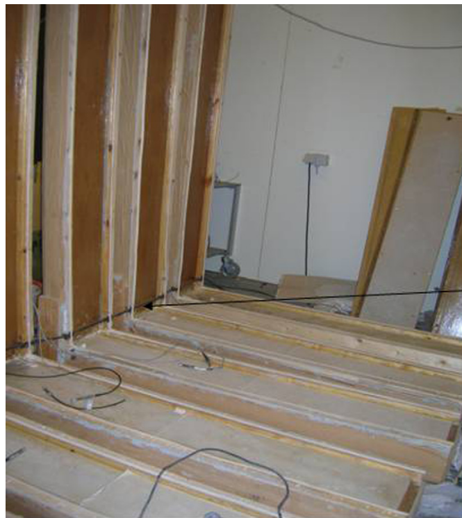
Fig. 1. The figure shows five of the six L-shaped test rigs, here open with the moistened gypsum boards inside. The arrow points to the heating cable T-18.
