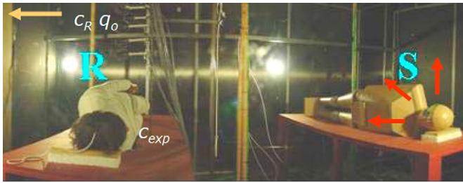
Fig. 1. Two patients (life-size manikins) in a hospital ward. The right patient is the source of airborne infection, and the left patient is the target.
