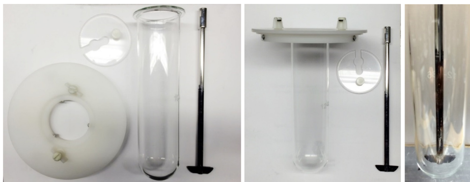
Fig. 1. Mini vessel dissolution apparatus, including the small volume vessel, mini paddle impeller, small lid, and the mounting plate to adapt the mini vessel to the standard opening for the USP 2 vessel in a typical dissolution testing system.
