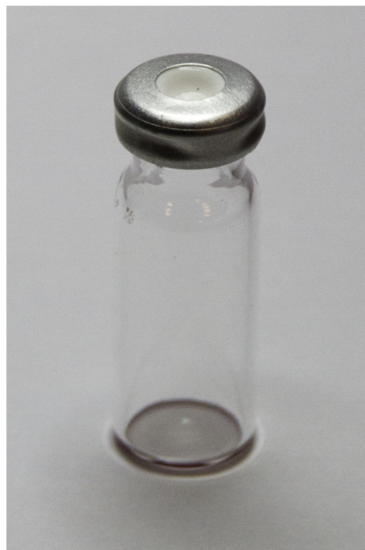
Fig. 1. Vacuum glass vial (ref 2C1702KD, Interchim).
