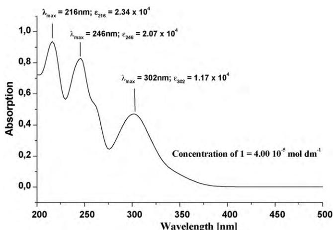
**Fig. 1.** The UV–vis spectrum of **1** in receptor solution.
