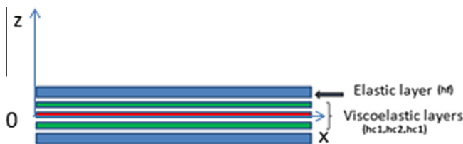
Fig. 1. Five layered sandwich beam structure.
