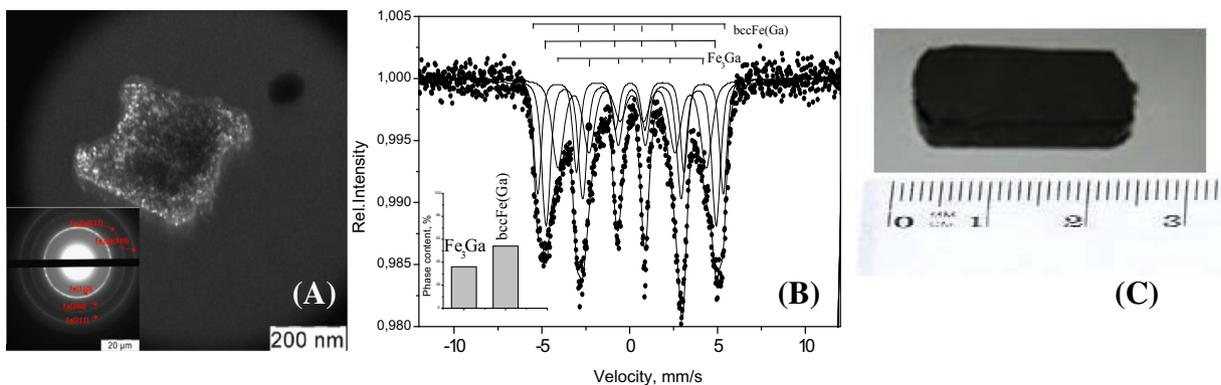
**Fig. 1.** Microstructure of synthesized FeGa-alloy particles: (A) dark field TEM image of the particle, (B) Mossbauer spectrum of synthesized particles with derived phase analysis (in inclusion), (C) real size of the FeGa/PU composite ( $x$  – the direction of applied magnetic field at manufacturing).
