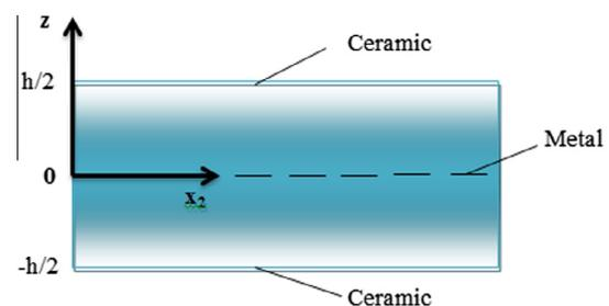
Fig. 1. The material characteristic of sigmoid functionally graded material.
