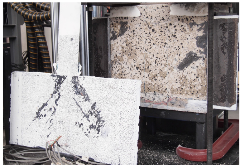
Fig. 1. Specimen testing rig details (a) configuration of test rig (front view); (b) Photograph of typical patch anchor debond failure.
