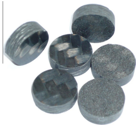
Fig. 1. Specimens for the creep compression tests.
