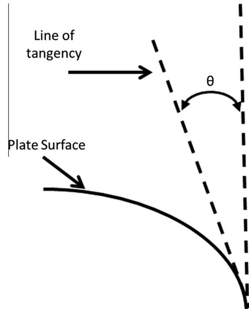
Fig. 1. Plate curvature measure definition.
