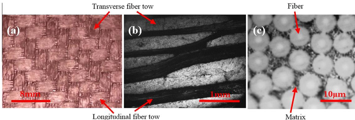
Fig. 2. Optical Micrograph of 2D C/C Composite (a) top surface (b) cross-section and (c) magnified cross-section.
