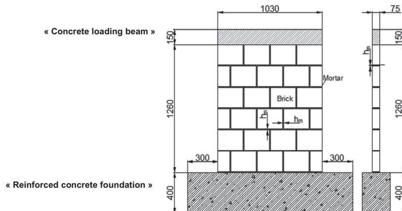
**Fig. 1.** Description of unreinforced masonry wall (reference).
