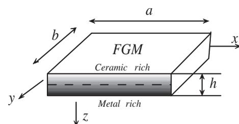
Fig. 1. Geometry and coordinate system of FGMs plate.
