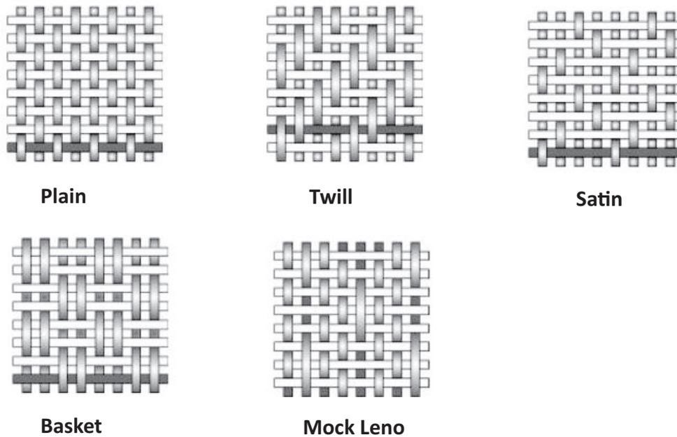
Fig. 1. Different configurations of woven composites.
