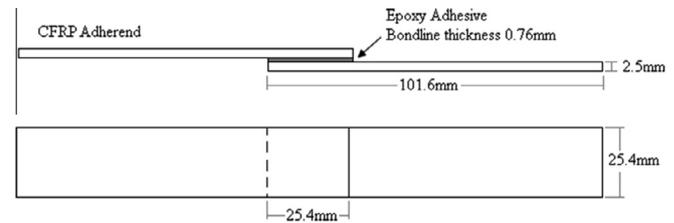
Fig. 1. CFRP-epoxy single lap shear joint.
