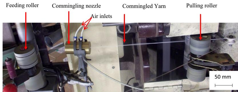
**Fig. 2.** Commingling yarn processing line in Composite Centre of The University of Manchester.
