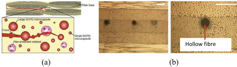
**Fig. 1.** Different healing concepts in composite structures: (a) insertion of microcapsules in a thermoset resin system [20] and (b) using hollow fibres filled with a healing agent [29].
