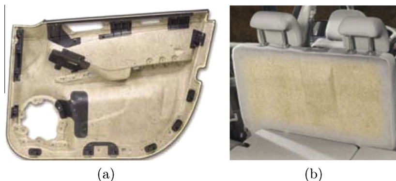
Fig. 1. Example of natural fibre composite parts for interior applications of a Mercedes vehicle [36].
