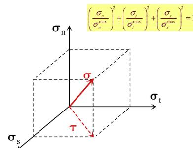
Fig. 4. Damage initiation criterion for the adhesive layer.
