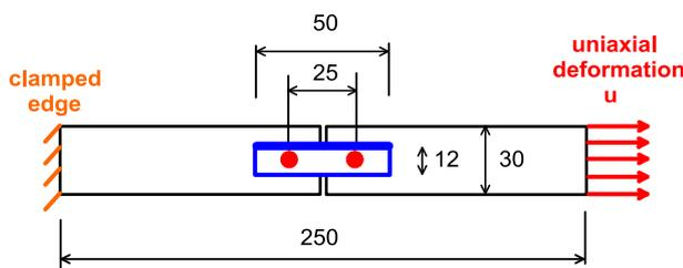
Fig. 2. Boundary condition for deformation of the hybrid joint.
