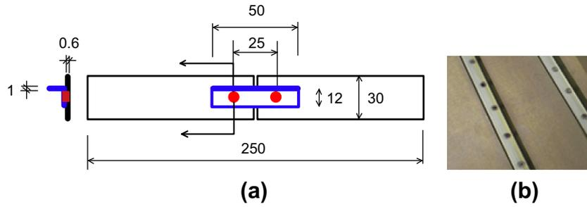
Fig. 1. Geometry of the sample.
