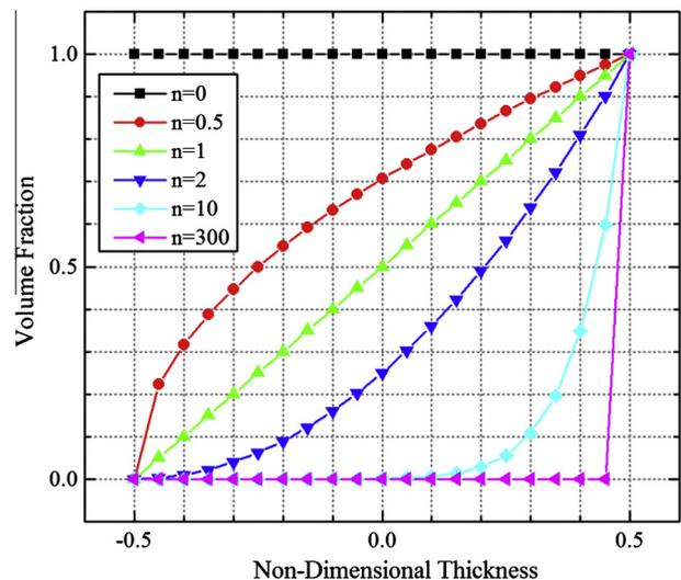
Fig. 1. Through-the-thickness variation of the ceramic phase volume fraction for different values of  $n$ .
