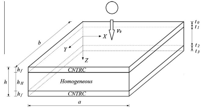
**Fig. 1.** Configuration of a carbon nanotube reinforced composite (CNTRC) laminated plate subjected to low velocity impact.
