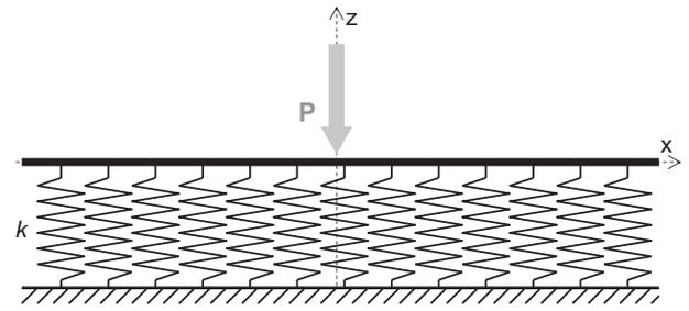
Fig. 1. Beam resting on one parameter Winkler elastic foundation.
