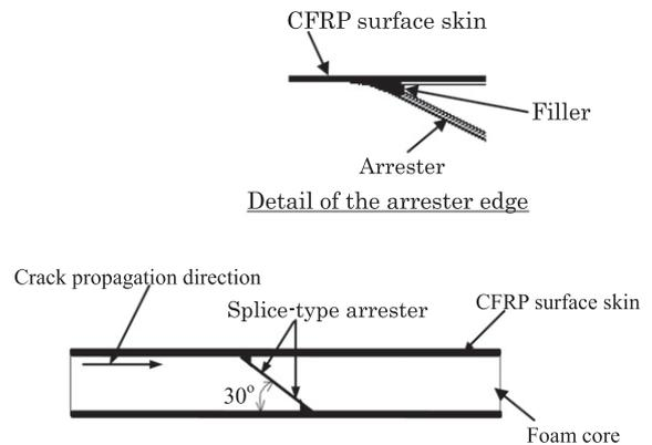
Fig. 1. Schematic diagram of splice-type arrester with filler.
