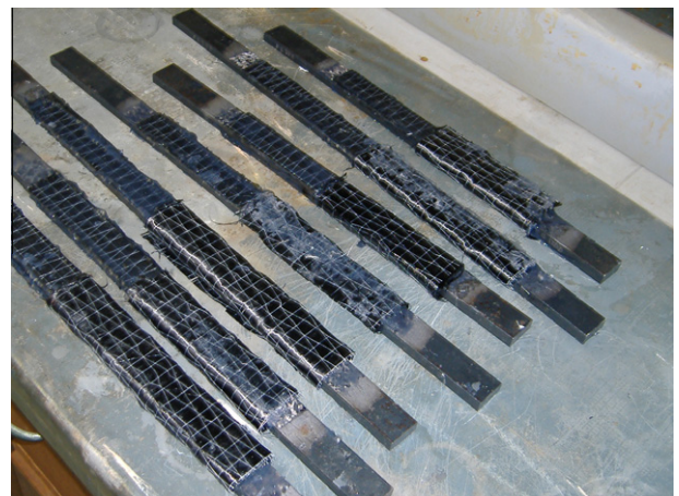
Fig. 2. Test specimens. (a) Double strap joint. (b) Single strap joint.
