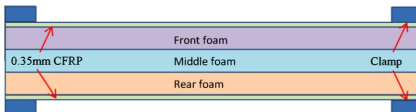
**Fig. 1.** Sketch of the stacking configuration of a graded foam sandwich panel.
