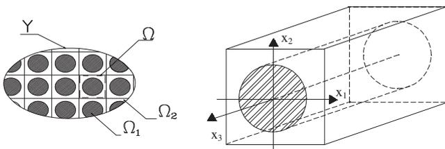
Fig. 1. Periodic fiber reinforced composite.
