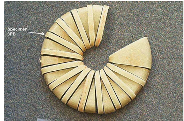
Fig. 2. Sectioning of hub disc prototype to obtain specimens for bending tests.
